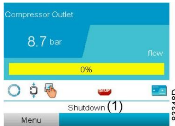
Typical display when the vacuum pump is stopped by a shutdown
