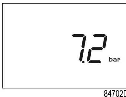
Main screen with pressure (stopped compressor)
