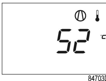
Main screen with temperature (stopped compressor)
