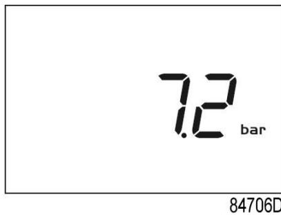
Main screen with pressure (stopped compressor)
